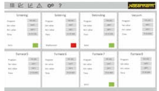
Clear display of connected furnaces
