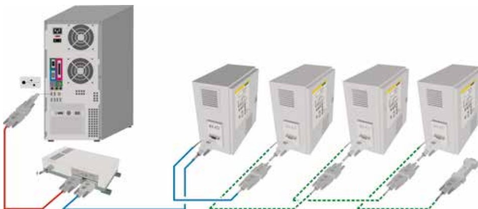
Extendable for connection of up to 16 furnaces
