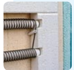
Heating elements mounted on carrying tubes
